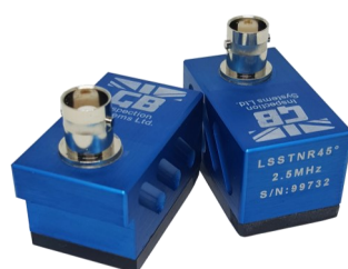
LSSTNR Available angle 45° Network Rail Approved Version Single Shear Wave for high angle scan. Crystal Size: 15mmø
